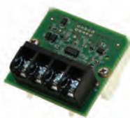
Fig. 12: Load Current Card (Accessory 23GA/GB)
