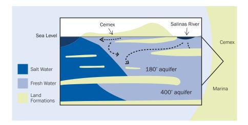
The third significant finding involves a major flaw with the test slant well, which is part of the proposed CalAm desalination plant. The Stanford Study confirmed that dredge pond operations at Cemex are mounding seawater, and due to this mounding, results from the test slant well are biased. The test slant well data is a flawed assessment of the ratio of seawater to freshwater.
